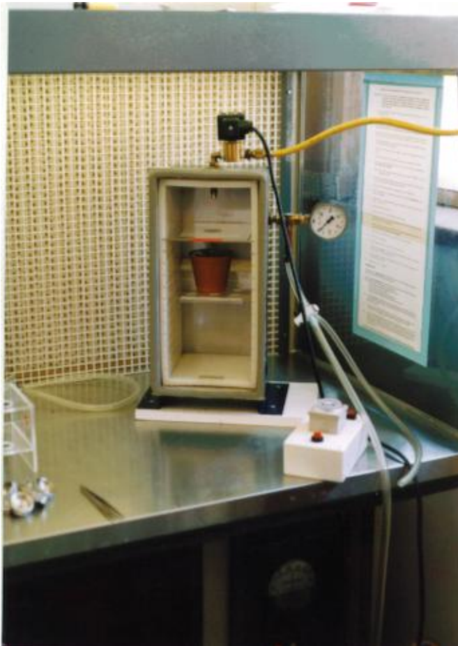
Figure 2.1. Particle bombardment device used in plant transformation experiments. Tissue is placed inside the chamber which is evacuated of air to form a partial vacuum. DNA-bearing particles are then accelerated into the plant tissue under the pressure of
